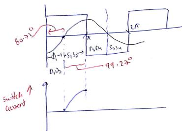
$$I_{1ms}^{2} = \left\{ \frac{1}{2\pi} \int_{0}^{2} 9^{2} \sin^{2} \omega t \right\} d\omega t$$
