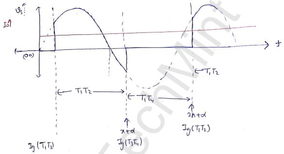
$$V_0 = \int_{0}^{\infty} V_0 \sin \omega t d\omega t = \frac{V_0 \cos \alpha}{T} = \frac{220\sqrt{5} \times \cos \alpha}{T}$$
