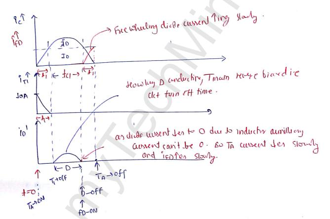
O For a vollage commutated they ckf shown in fig cap' is initially Charged to Vs valtage with polarity shown in Rig Find the let turn oft time of main thyristr
