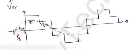
$$C_n = \frac{6x}{m\pi} = \frac{6 \cdot v_{5/2}}{m\pi} = \frac{3v_5}{m\pi}$$
