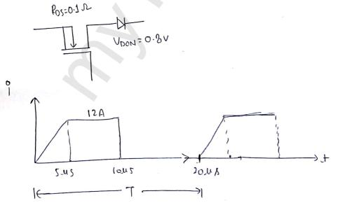
Find the power loss in the mostet and the diche in a composite switch.
